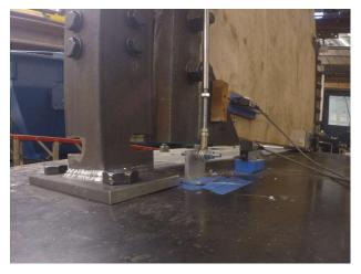
Figure 9. Rocking and gap-opening mechanism at 3% drift
