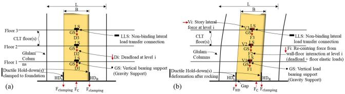
Figure 1. System Level Mechanics (a) Core loads: Dead Load Case (b) Core Loads: Re-Centering + Earthquake Case
