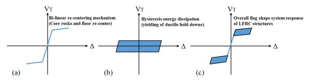
Figure 2. System Response (a) Re-centering mechanism (b) Hysteresis energy dissipation (c) Overall LFRC system response
