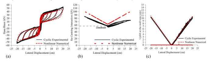
Figure 8. Results from cyclic test and nonlinear numerical analysis a) Lateral Force vs Displacement b) Floor Re-centering Interaction vs Displacement c) Uplift at the wall toe (hold-down elongation) vs Displacement
