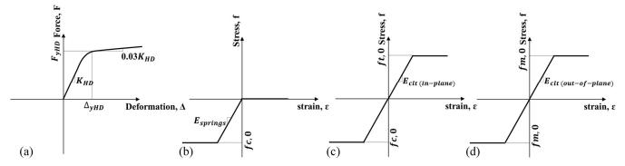
Figure 5. Material behavior of structural elements a) Hold-Downs b) Compression-only Zero Length Springs c) CLT wall inplane loading action d) CLT floor out-of-plane loading action
