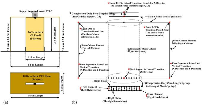
Figure 4. LFRC example for numerical analysis (a) The geometry of the model (b) Numerical model of the system
