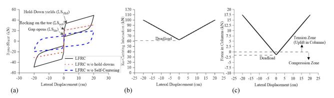
Figure 6. Results from cyclic numerical analysis a) Base-shear vs drift b) Floor Re-centering Interaction vs drift c) Force in Columns vs drift
