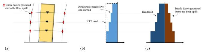
Figure 3. Internal Load Distribution (a) Schematic of the structure deformation (b) Core axial load (c) Column axial load
